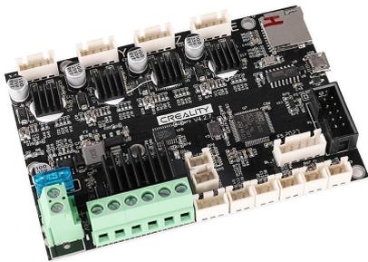
The first part that we are going to upgrade is going to be the motherboard. Most Enders come stock with a 4.2.2 motherboard. This is going to be the first thing that we swap out, the biggest difference between these two boards is that the 4.2.7 is a 32 bit board and it also come equipped with silent stepper drivers. This means that your printer will produce less noise and not annoy your partner whenever it is running.
