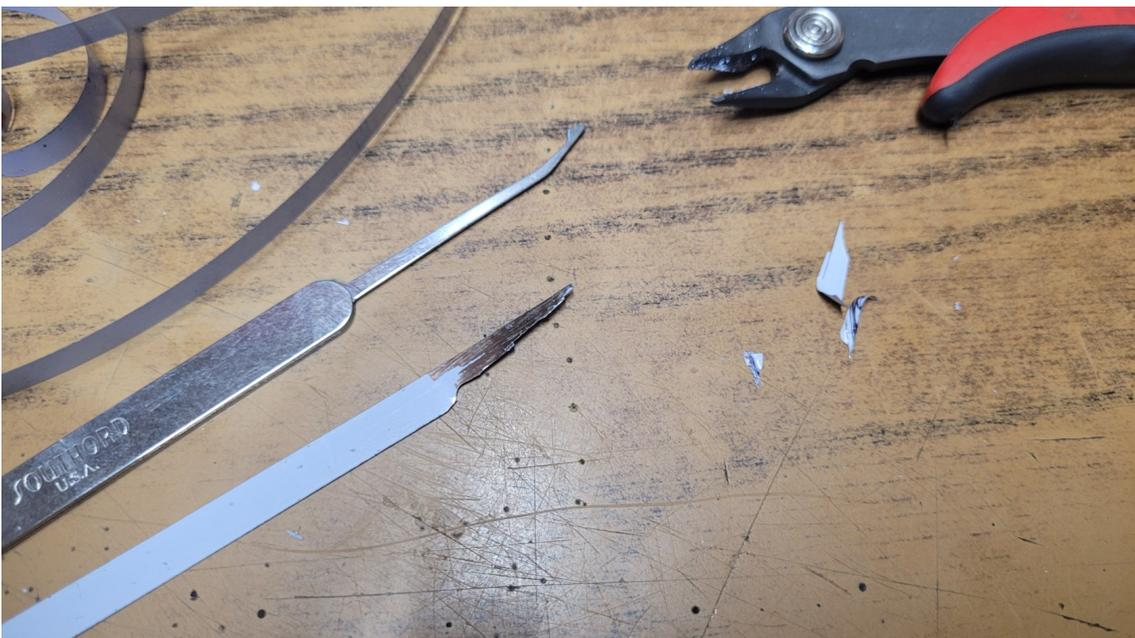
In the end I used the kitchen shears to cut an angle on the other end, and a cheap diamond file to smooth out the edges and burrs (sandpaper is great too!)
