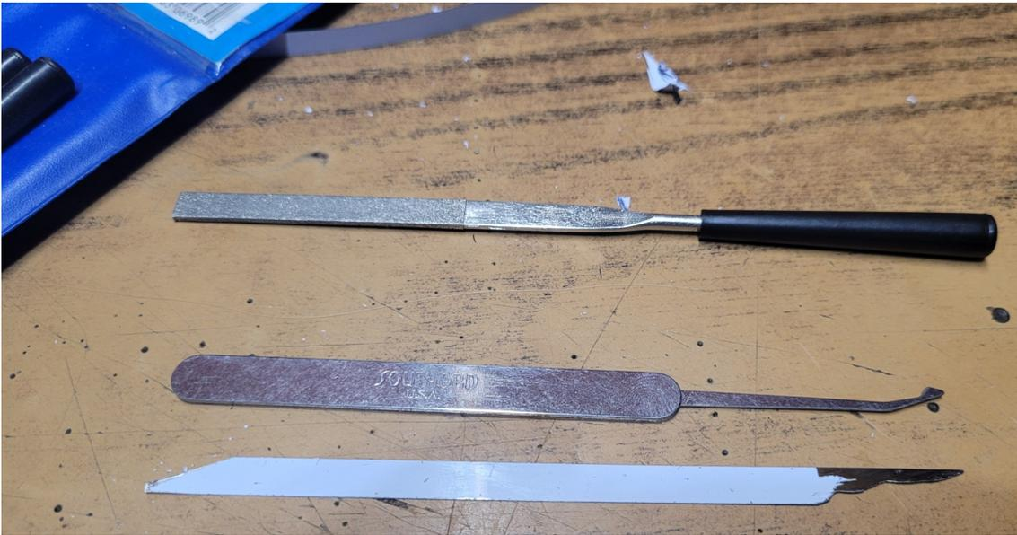
Leaving the paint (or powder coat) on the tape it measures 0.0035" (or 35 ten-thousandths of an inch, or 0.089mm, or 89 microns thick), and when I scrapped the coating off it measured an even 0.003" (or 3 thousandths of an inch, or 0.076mm, or 76 microns). This size is very thin and great for the more delicate tasks (decoding mostly), but less good for the harsher tasks. (bypassing master 175s)
