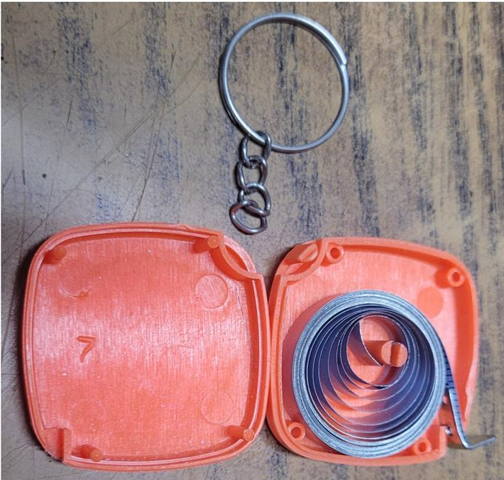
I used a cheap pair of flush cutters to chop off the tightest curled part (at less than \$3 for the whole tape, it wasn't worth the extra effort to straighten)
