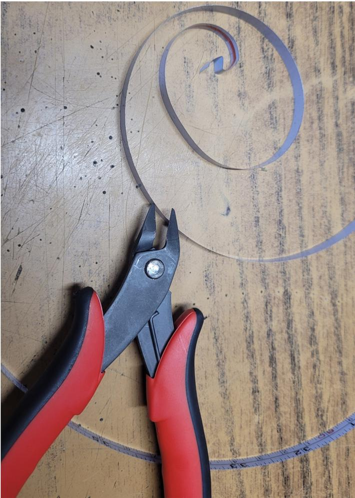
Butchering the tip to make a slimmer end was a ton more trouble than expected... Since the metal tape is hardened, it tends to break rather than cut with these cutters (Lesson - kitchen shears or tin snips work way better!)
